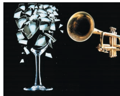
A singer or musical instrument can shatter a crystal goblet by matching the goblet’s natural oscillation frequency.
