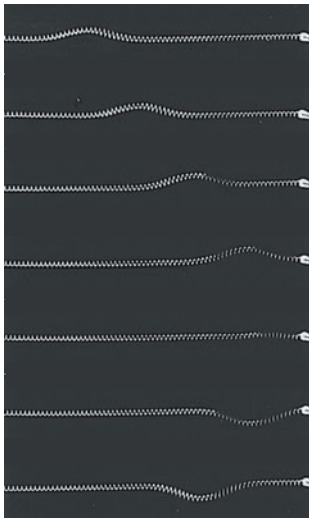
FIGURE 21.9 A strobe photo of a pulse traveling along a rope-like spring.
