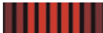
Interference fringes in an optical double-slit interference experiment.
