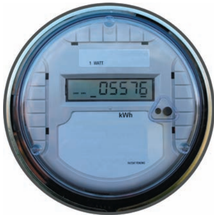
The electric meter on the side of your house or apartment records the kilowatt hours of electric energy that you use.
