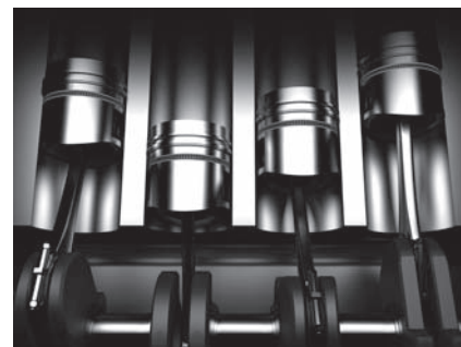
The pistons in a car engine do work on the air-fuel mixture by compressing it.
