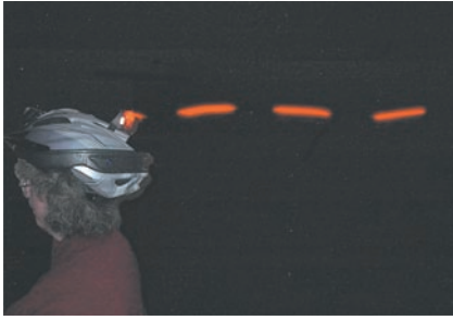
The rear flasher on a bike helmet flashes on and off. The timing is controlled by an RC circuit.
