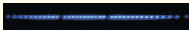
FIGURE PSVII.2 This string of beryllium ions held in an ion trap is being studied as a possible quantum computer. The quantum states of the ions are manipulated with laser beams.
