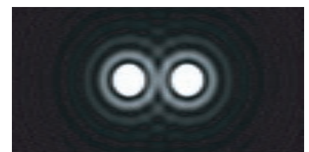
FIGURE 24.19 Enlarged photographs of the images of two point sources.
