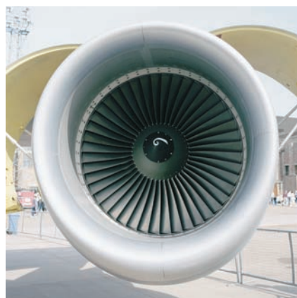
A jet engine uses a modified Brayton cycle.
