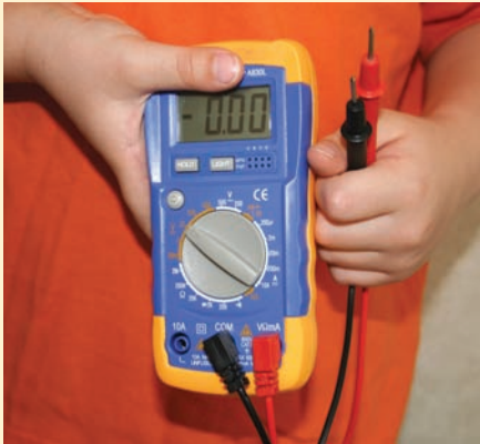
■ FIGURE 5.34 A handheld digital multimeter.
