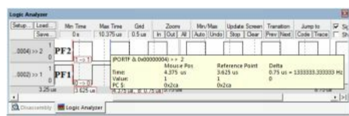
Figure 4.17. Logic analyzer in the Keil uVision simulator measures the frequency of the squarewaves.
