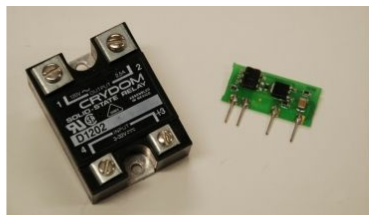
Figure 8.17. Solid state relays can be used to control power to an AC appliance.
