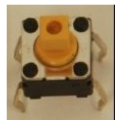
Figure 2.8. Single Pole Single Throw (SPST) Switch interface. The photo is a B3F tactile switch.
