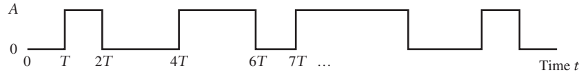
FIGURE 10.2 Example of binary PAM transmission with on-off signaling; T denotes symbol interval.
